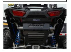
6. Install rear Gibson beauty plate. Use the factory bolts and supplied nylock nuts for the top two holes. Once they have been installed tighten the Gibson brackets at the rzr frame. Adjust plate for a level finish.
