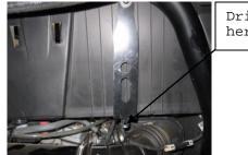
3. Next use a ¼" drill bit to drill the hole for the tailpipe brackets. You will drill the lower threaded hole on the both driver and passenger side rear bed bracket. See above photo for location. Drill hole on both sides of the vehicle.
