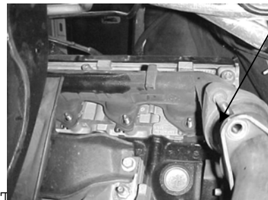
#6. FACTORY FLANGE CONNECTION. DISCONNECTING POINT.
