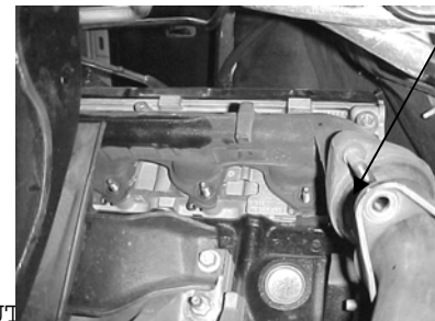
#6. FACTORY FLANGE CONNECTION. DISCONNECTING POINT.
