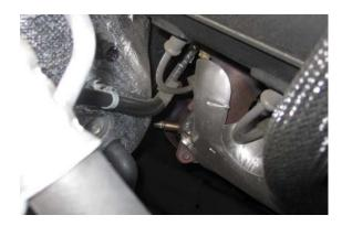
8) REMOVE THE FIVE BOLTS ATTACHING THE MANIFOLD TO THE HEAD. REMOVE THE MANIFOLD FROM THE TOP OF THE VEHICLE.CLEAN THE SURFACE OF THE HEAD. REMOVE ANY CARBON DEPOSITS THAT MAY BE ON THE HEAD.PREPARE THE SUPPLIED HEADER BOLTS WITH ANTI-SEIZE TO THE THREADS.
