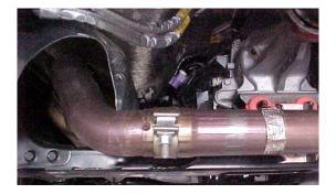
5. DISCONNECT ALL O2 SENSORS. THEN FROM UNDERNEATH THE VEHICLE, LOOSEN THE
