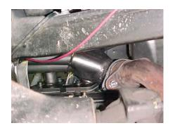
YOU MUST RE-TORQUE YOUR HEADER BOLTS APPROX. 100 MILES AFTER INSTALLATION. IF NOT DONE THE HEAD GASKET WILL LEAK AND IS NOT COVERED UNDER WARRANTY.
