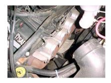
4. ONCE THE DRIVERS SIDE MANIFOLD IS REMOVED USE A WIRE BRUSH TO CLEAN HEAD SURFACE. INSTALL SUPPLIED DRIVER SIDE HEADER, GASKET AND HARDWARE. TORQUE HEADER TO 30 TO 35 FTS. AFTER DRIVERSIDE HEADER IS INSTALLED PUT SUPPLIED HEAT WRAP ON SPARK PLUG WIRES #7 AND 9 FOR HEAT PROTECTION. RE-INSTALL AIR CLEANER ASSEMBLY.
