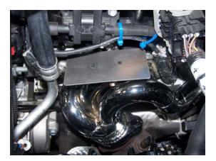
4. (NOTICE IN PICTURE) THERE IS SUPPLIED HEAT SHIELD TO BE CLAMPED ON MIDDLE HEADER TUBE. THIS WILL PREVENT HEAT GOING TO COIL PACK ABOVE HEADER ASSEMBLY. NOW RE-INSTALL STEERING SHAFT USING RED LOCKTITE BEFORE TORQUING FASTENER.
