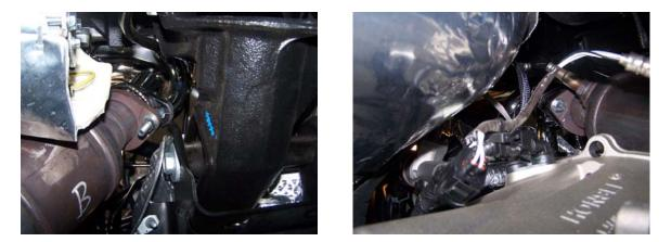
8. PERIODICALLY CHECK AND RETIGHTEN THE HEADER BOLTS.
