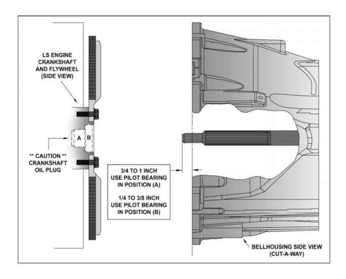
**Pilot bearing for crankshaft position "A"** is a **SMALL** outside diameter (1.094") <u>GM pilot bearing</u> that fits into the innermost pocket of the crankshaft flange. This bearing is typically (but NOT ALWAYS) used with Transmission/Bell housings on GM; LS1 powered vehicles from 1998 to 2002. NOTE: if using the small GM pilot bearing, the internal O-ring seal faces the transmission when installed properly.
