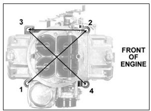
Figure 2—Carburetor torque sequence (all Holley carburetors)
