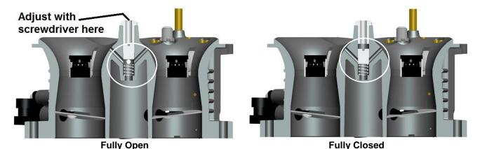
The idle bypass valve allows for additional airflow through the carburetor, while maintaining the desired relationship between the throttle plate and the transfer slot. Applications using a larger cam may benefit most from this new feature. This valve replaces the need for holes in the throttle plates.
