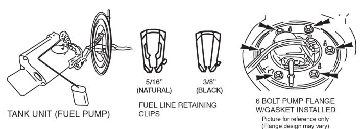
NOTE: This tank unit may look different than the O.E. unit. This replacement unit meets all specifications established by the O.E. manufacturer. It will fit and function properly if all the installation procedures outlined in this instruction sheet are followed.
