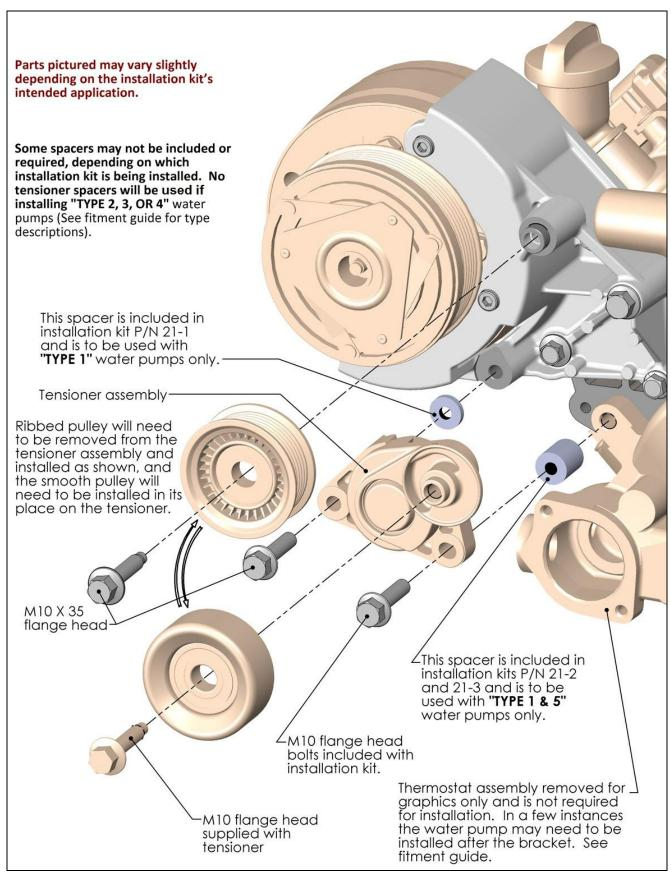
NOTE: Torque M8 bolts to 18 ft./lbs. and M10 bolts to 36 ft./lbs.
