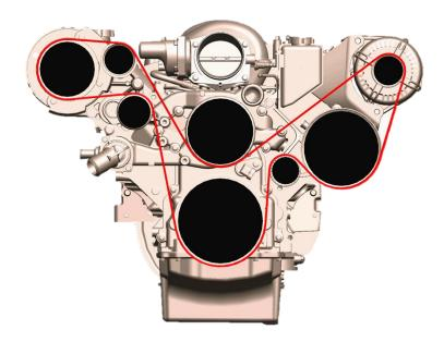
**HELPFUL HINT:** When installing the belt, route around all the pulleys except the water pump pulley. While fully rotating the tensioner arm, slip the belt on the smooth water pump pulley last.
