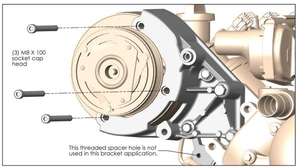
NOTE: Torque M8 bolts to 18 ft./lbs. and M10 bolts to 36 ft./lbs.
