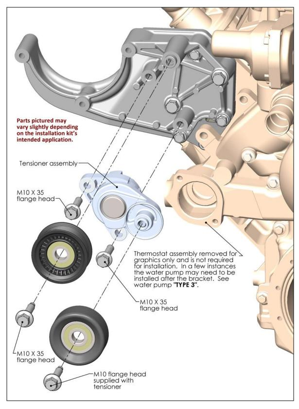
**NOTE:** Torque M8 bolts to 18 ft./lbs. and M10 bolts to 36 ft./lbs.
