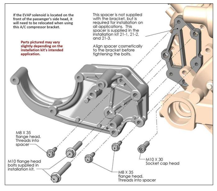
NOTE: Torque M8 bolts to 18 ft./lbs. and M10 bolts to 36 ft./lbs.
