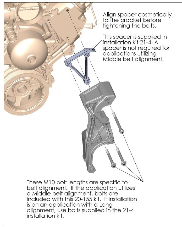
**NOTE:** Torque M8 bolts to 18 ft./lbs. and M10 bolts to 36 ft./lbs.
