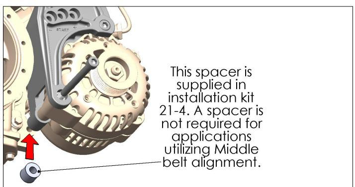
**NOTE:** Torque M8 bolts to 18 ft./lbs. and M10 bolts to 36 ft./lbs. **Helpful hint:** When wiring the alternator, install the included 197-400 plug into the alternator. Next connect the yellow wire to switched voltage that is "on" when the key is in the run position. If the vehicle has a "charge indicator light" the yellow wire can be connected to that circuit.
