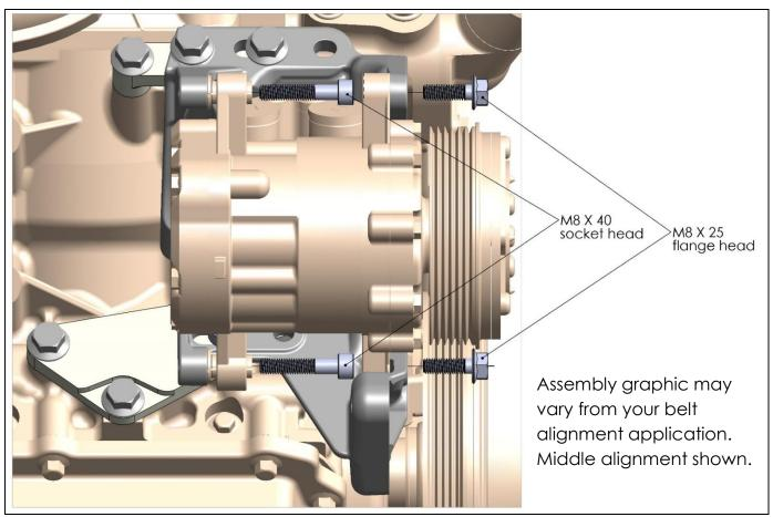
Torque M8 bolts to 18 ft./lbs. and M10 bolts to 36 ft./lbs.
