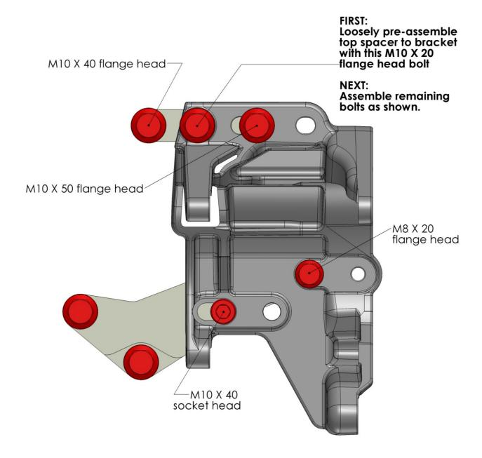
At this time torque M8 bolts to 18 ft./lbs. and M10 bolts to 36 ft./lbs.
