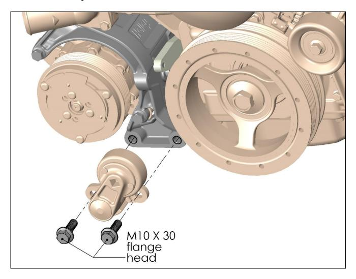
Torque M8 bolts to 18 ft./lbs. and M10 bolts to 36 ft./lbs.
