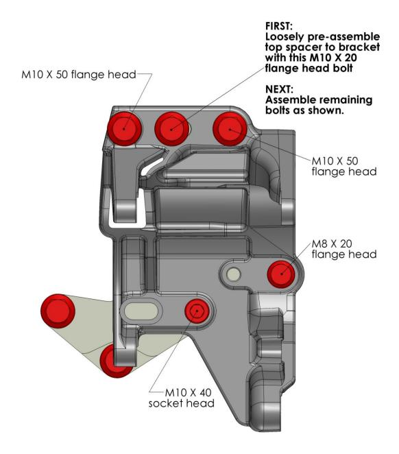
At this time torque M8 bolts to 18 ft./lbs. and M10 bolts to 36 ft./lbs.
