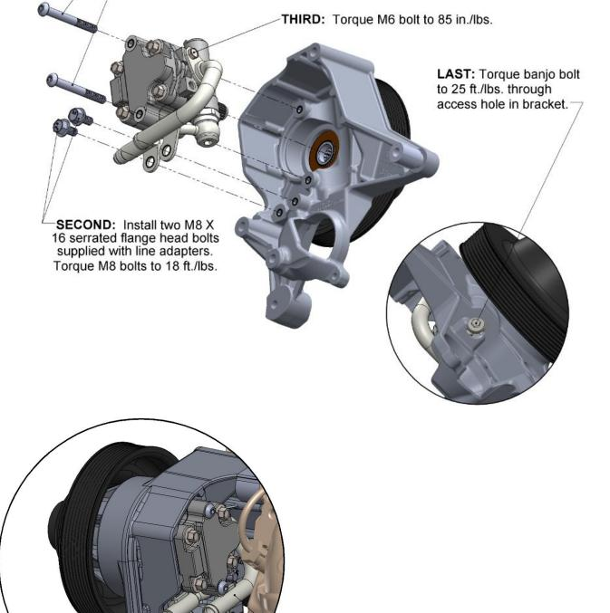
**NOTE:** It may be desirable to install the pump feed hose before installing the bracket assembly to the engine. Access to the tube may be difficult after assembly **especially** on dry sump applications.
