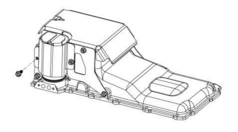
**NOTE:** Starting with the bolt, torque fasteners to 18 ft./lbs.
