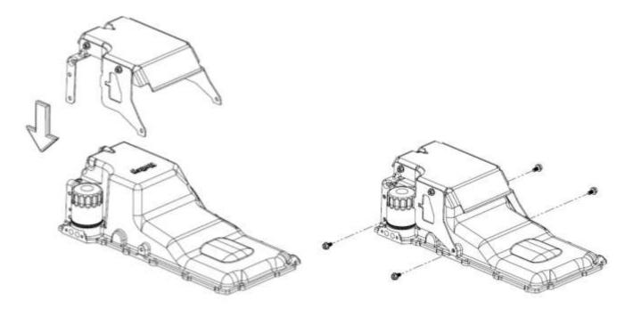
**NOTE:** Starting with the bolts and then the nuts. Torque fasteners to 18 ft./lbs.
