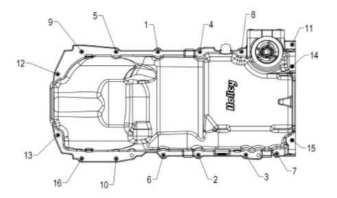
Torque: M8 bolts to 18 ft./lbs. (bolts 1 through 13, and 16) M6 bolts to 106 in./lbs. (bolts 14 and 15)
