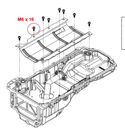
Reinstall the windage tray. Apply a drop of blue Loctite® to the threads of the supplied (x7) M6 x 12 flange head bolts. Install the (x1) M6 x 16 flange head bolt in the location that also goes through the pickup tube bracket. Torque the bolts to 10 ft./lbs.
