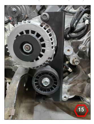
6. Inspect the assembly and ensure all hardware has been torqued to the proper specification. A longer belt is required since the alternator position has moved. Holley recommends using a **6PK2250**. This belt can be found at most automotive parts retailers. Below is the proper belt routing.
