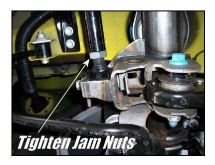
You are now finished with the installation of your new Hotchkis Adjustable Panhard Rod. Double check to make sure all hardware is fully tighten before driving the vehicle.
