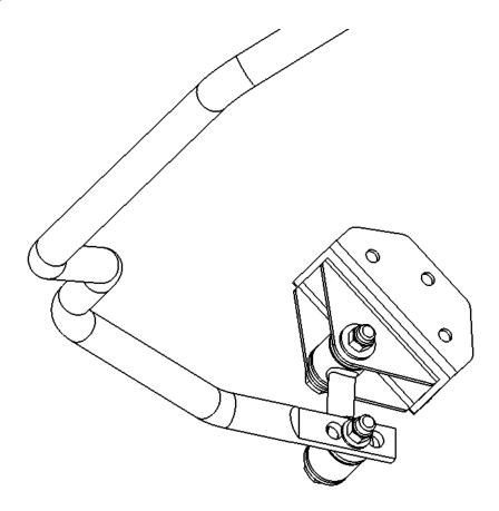
4R Rotate sway bar, and frame brackets up until they contact the frame rails. (Fuel lines, and parking brake cables may need to be loosened, and moved for proper placement of frame brackets, and can be re-installed when finished.)
