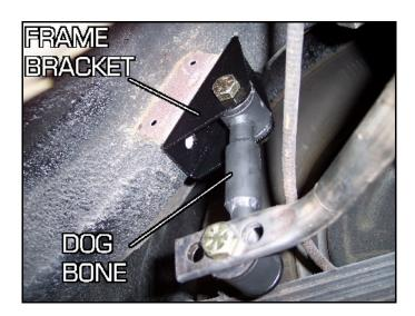
We've noticed on some E-bodies that the distance between the left and right frame rails were ½" wider. If the frame bracket does not line up in the center of each frame rail due to the frames having a wider span, then please install the optional spacer between the sway bar and the end link.
