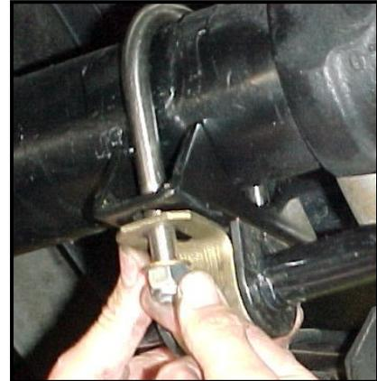
With the bar hanging freely you can slide the u-bolts along the axle until the bar is centered with the vehicle. Tighten down the nuts on the u-bolts to secure the position of the u-bolts and brackets.
