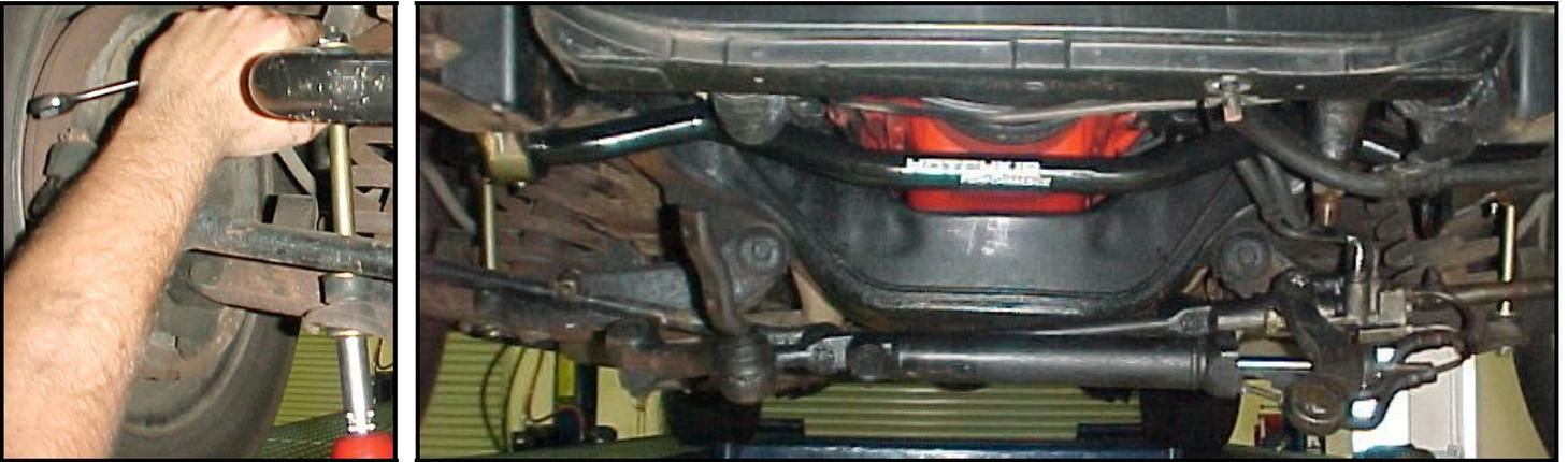
For cars without a stock front bar, you will have to connect the end links to the sway bar. Attach the end link mount bracket included with the kit to the end links and tighten. Rotate the full assembly into position against the lower a-arm and drill the mounting holes in the arm. Use the 10mm bolts from **hardware kit #T1711** to secure the brackets.
