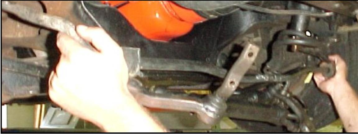
*Leave the steering loose for installation of the Hotchkis sway bar at a later step.*
