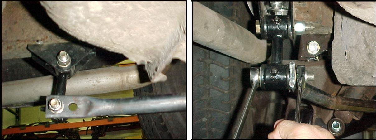
You can also adjust the stiffness of the bar by changing the hole the end link mounts to. The hole nearest to the end of the bar softens the bar stiffness by lengthening the bar. The hole furthest from the end of the bar stiffens the bar by shortening the length of the bar.
