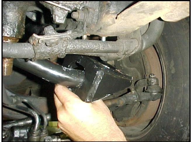
Tighten the hardware on the inside edge of the bracket nearest to the hole that the bar passes through.
