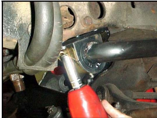
*The driver's side bracket mounts inside of the power steering bracket included with the Hotchkis kit. Slide the retainer bracket into place over the bolts and tighten the bracket into place.*
