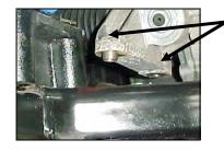
2 bolts per side; allows more open space without pulling on firewall grommet.
