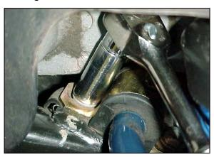
Now, remove the sub-frame hardware. Using a 16mm socket, remove the 2 bolts (1 per side) located just forward and up of the brake line and sensor - shared bracket. The other 2 (again, 1 per side) are located just inboard. You'll see one just above the stability sensor on the left upper link.
