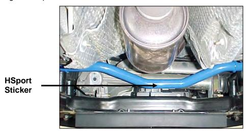
10/ Once the HSport bar is positioned, grease the inner portion of the two supplied front bushings (1/4 of the tube for each). Then, install the bushings over the bar on the outside of the washers as shown.
