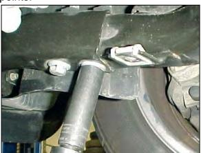
5/ That's it for the sub-frame. Now you must disconnect the lower motor mount. Using the same 16mm socket, or a wrench, remove the horizontal bolt. Then, remove the vertical bolt as shown.
