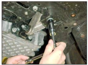
6/ Before removing the front anti roll bar bracket bolts, we highly recommend you remove the four steering rack bolts. Not required but if the sub-frame is pulled down with the rack still attached, this may pop the rubber grommet from the firewall. Removing the four bolts is time consuming but so is reinstalling the grommet – you choose! Use a torx (E 12) socket or wrench.
