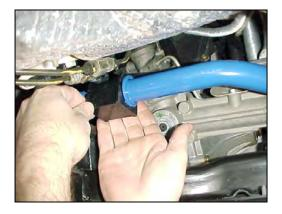
11/ Then, install the larger supplied bushing brackets over the bushings with the grease fittings facing inwards or towards each other.
