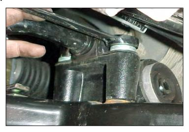
8/ Finally, the bar is free and you are ready to remove it. Do this by simply rotating the center to lift the ends over the steering arms, then pull straight out towards the rear of the vehicle. You may have to maneuver the bar to better position it as it comes out but be patient.
