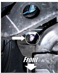
d) Finally, using the same 16mm socket, remove the 4 bolts (2 per side) at the front of the sub-frame where it slips into the two solid frame points.
