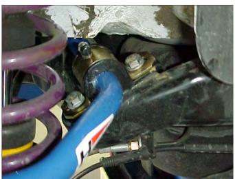
9/ Now, reinstall the 4 sub-frame bolts, bushing bracket bolts, spring/shock assemblies and end–links. Start the end links in the middle position and tune from there. Make sure all hardware is secure and tight.
