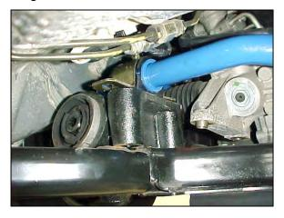
12/ Now, start with the bushing bracket bolts, then the steering rack torx bolts and reinstall all the rest of the sub-frame hardware. **Make sure ALL bolts are reinstalled and that they are tight and secure!**
