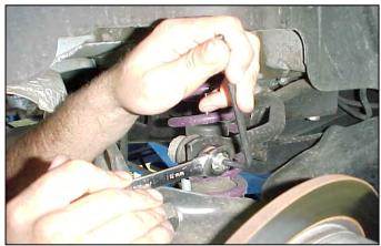
4/ Next, remove the two-spring/shock assemblies (only one side is required but both removed makes the job easier) using a 13mm socket with extension for the two upper bolts and a 21mm socket for the lower bolt as shown.
