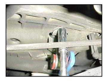
12) Use the new hardware to attach the end link to the sway bar. See below. The rear sway bar stiffness is 2-way adjustable. The hole closest to the end of the bar is the softest of the 2 settings.
