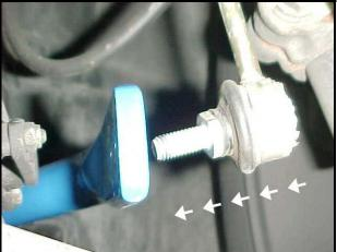
7) Install the subframe mounts back onto the vehicle. Use the provided spacer plate for each mount. Fully tighten all hardware at this time (including the endlink bolts!)
