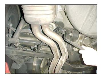
You will be reusing the stock end links for your new Hotchkis sway bar, so you will have to detach the end link from the bar. Soak the bushing down with some penetrating oil. Next, use a ball joint remover or similar tool to push the bar end through the bushing. Then remove the bushing.
