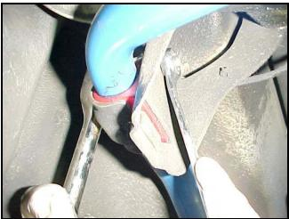
11) Install end links back onto the upper control arms
