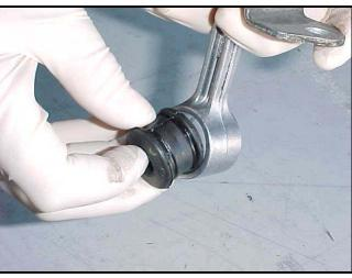
6) Lube your new polyurethane end link bushings and sleeve with the provided grease. Install the bushings and sleeve as shown.
