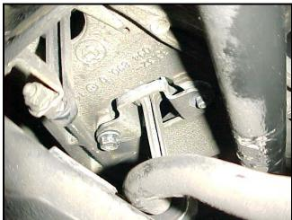
4) The sway bar should now be loose from the vehicle. You will have to fish one end past the exhaust pipes in order to remove the bar completely.
