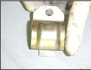
8) Lube the inside of your new polyurethane bushings and install them onto your Hotchkis Bar. At this time, you may install the bracket onto the bushing.
