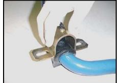
6) Reinstall the bar in the same manner as removal. Attach the end links to the sway bar. Do not fully tighten the end links at this time. You will notice that there are 3 hole settings: normal, medium, and stiff. The hole closest to the end is the normal setting. Choose the stiffness setting that suits your driving needs.
