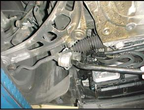
5) Apply the provided grease to the new polyurethane bushings. Install the new bushings onto your new H-Sport sway bar. At this time you may also install the bushing bracket.
