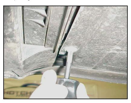
Loosen the end link nut, leaving it on it's last couple of threads. The end links will hold the sway bar for you while you unfasten the subframe mounts described in the next step. Once the subframe mounts are detached, then you can spin off the end link nuts quickly allowing you to remove the sway bar easily.
