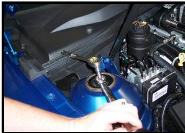
6. Mark the strut where the upright nuts are located with a marker. Remove the bolts that hold the spindle to the strut.
