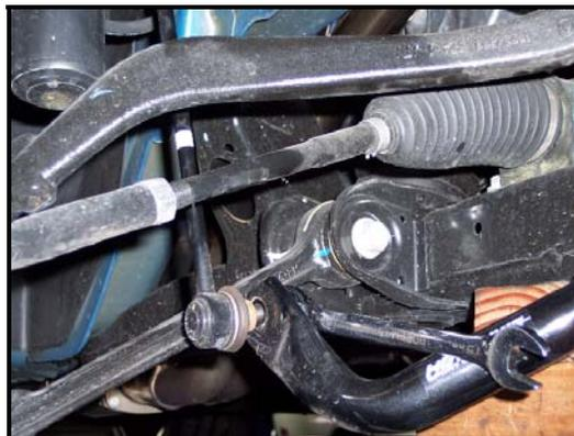
3. Disconnect the OE end link from the front struts. Retain the nut for reinstallation.
