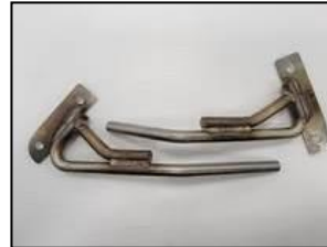
Rear over-axle hangers
