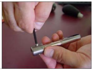
**STEP 15.** Move the stick to the "Park" position and thread the Hurst stick down as far as possible making sure there is no interference with the Hurst plate. The set screw should face towards the front.
