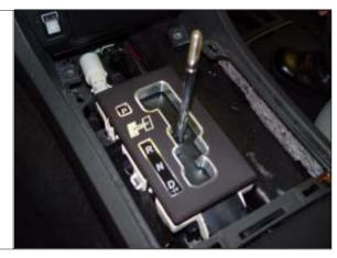
**STEP 14.** Start the set screw into the threaded hole on the front of the HURST stick.
