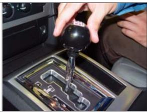
**STEP 20.** Tighten or "jam" the large nut up against the Hurst knob while holding the knob with the correct logo orientation.
