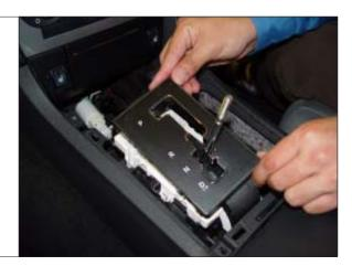
**STEP 9.** Remove the black plastic slider from the shift stick by pulling upwards. Take note of where the nub on the slider is located. The nub is commonly found at the bottom of the slider. Bend the ends of the slider aggressively, creating creases.
