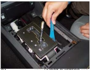
**STEP 8.** With the tabs on the passenger side free, lift up on the black plastic shifter plate and move it towards the driver's side to free it from the tabs on the left hand side.
