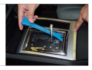
**STEP 5.** Remove the black rubber tray in front of the shifter by sliding it up and out. Then remove the two screws that are under the rubber tray.
