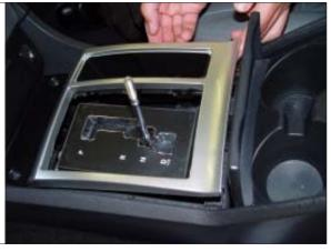
**STEP 7.** Remove the black plastic shifter plate by prying the tabs on the passenger side (front and back) from the white shifter housing.
