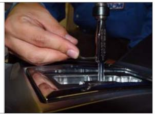
**STEP 19.** Carefully screw the HURST knob all the way down until it contacts the large jam nut, then unscrew the knob until the logo is aligned correctly.
