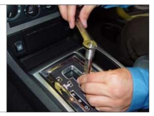
**STEP 18.** After the HURST stick has been "jammed" with the M8 jam nut and you have made sure that the stick is straight, tighten the set screw on the front of the stick to ensure that the Hurst stick is securely attached to the original shift stick.
