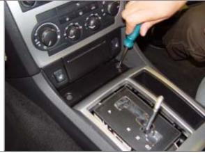
**STEP 6.** Gently remove the surrounding plastic cover by pulling upwards to access the tabs that secure the OEM plate to the white shifter housing.
