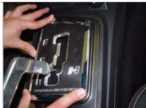
**STEP 22.** With the key in the ignition (vehicle "OFF") and foot firmly depressing the brake pedal, cycle the shifter through all positions to ensure smooth and accurate movement. If binding or rough movement occurs, review and ensure that STEP 9 & 10 has been completed or needs to be revisited.
