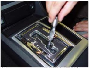
**STEP 16.** Thread the large Jam Nut to the HURST stick all the way down towards the end of the threads to make space for the M8 jam nut and the Shift Knob.
