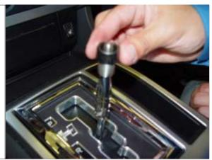
**STEP 17.** Thread the M8 Jam Nut onto the top of the stock stick and tighten with a wrench while firmly holding the HURST stick to prevent it from rotating.
