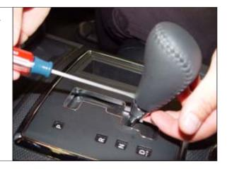
**STEP 3.** Remove the knob by unscrewing it from the stick. Remove the collar after removing the knob.
