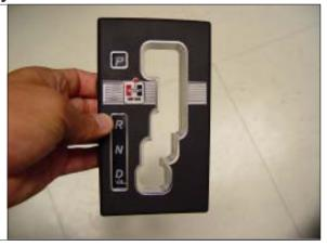
**STEP 13.** To attach the HURST plate, align the right side slots in the plate with the tabs on the white shifter housing, then push down on the left side of the plate to snap into the tabs on the left side.
