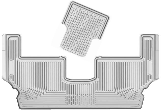
TO INSTALL YOUR LINER IN A PACIFICA WITH  $2^{\rm ND}$  ROW BUCKET SEATS, FIRST SLIDE BOTH 2ND ROW SEATS FORWARD TO ALLOW EASIER ACCESS TO THE 3RD ROW FLOOR. WITH THE SEATS MOVED, INSTALL THE LINER POSITIONED AS SHOWN ABOVE. NOTE THAT THIS LINER ONLY WORKS WITH  $2^{\rm ND}$  ROW STOW-N-GO SEATS. (OVER)
