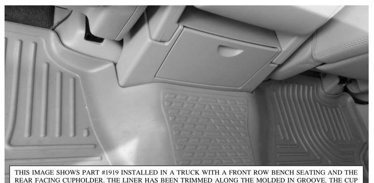
HOLDER IS FULLY FUNCTIONAL. A UTILITY KNIFE OR HEAVY SHEARS WORK WELL FOR TRIMMING.
