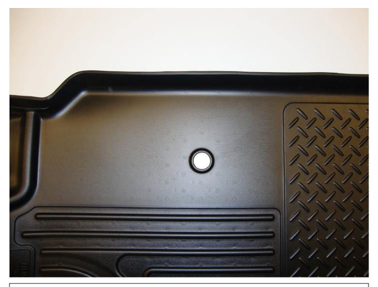
PART #9839 SHOWN TRIMMED FOR THE INSTALLATION OF THE JACK TOOL POUCH ON TOP OF THE LINER. TO TRIM, SIMPLY REMOVE THE MATERIAL FROM THE TOP OF THE RAISED BOSS AS SHOWN. IF YOU DO NOT HAVE A JACK TOOL POUCH OR PREFER TO NOT TO TRIM THE LINER, SIMPLY INSTALL THE LINER AS IT IS BOXED.
