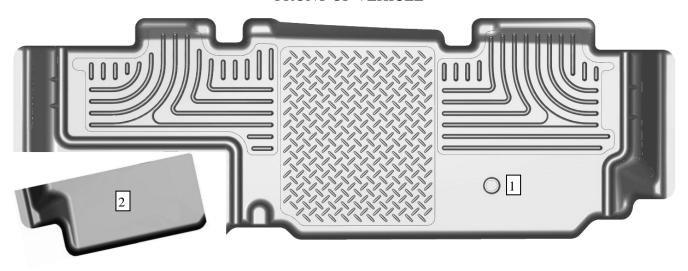
TO EASE INSTALLATION OF YOUR SECOND SEAT SUPER CAB FLOOR LINER, FIRST MOVE THE FRONT SEATS TO THEIR MOST FORWARD POSITIONS. WITH THIS DONE, INSERT LINER IN VEHICLE THEN REPOSITION THE FRONT SEATS AS DESIRED.
