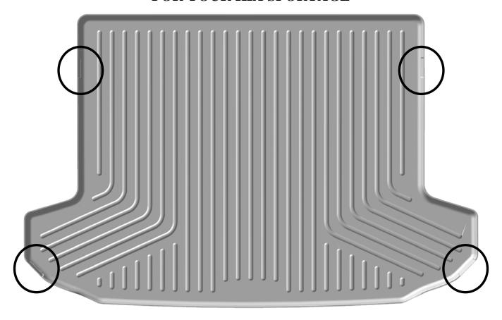
YOUR SPORTAGE HAS FOUR (4) CARGO TIE DOWN HOOKS LOCATED AROUND THE PERIMTER OF THE CARGO AREA. TO ACCESS TO THE FACTORY TIE-DOWN HOOK LOCATIONS (SHOWN CIRCLED ABOVE) WITH THE LINER IN PLACE. SIMPLY REMOVE/TRIM THE MATERIAL FROM THE PORTION OF THE LINER OVERLAPPING THE HOOKS. THESE AREAS ARE RECESSED ON THE LINER TO GUIDE TRIMMING. A UTILITY KNIFE WORKS WELL FOR TRIMMING.
