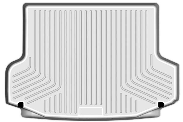
YOUR TUCSON HAS TWO (2) CARGO TIE DOWN HOOKS LOCATED AT REAR OF THE CARGO AREA. TO ACCESS TO THE TWO (2) FACTORY TIE-DOWN HOOK LOCATIONS WITH THE LINER IN PLACE. SIMPLY REMOVE/TRIM THE MATERIAL FROM THE AREAS OF THE LINER LOCATED DIRECTLY ABOVE THE HOOKS (AREAS ARE SHOWN DARKENED IN THE DIAGRAM ABOVE). THESE AREAS ARE RECESSED ON THE LINER TO GUIDE TRIMMING. A UTILITY KNIFE WORKS WELL FOR TRIMMING.
