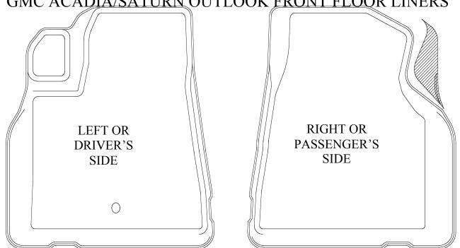
DUE TO DIFFERING DESIGNS OF THE PASSENGER SIDE KICK PANELS AVAILABLE IN THE ACADIA, ENCLAVE AND OUTLOOK, YOUR PASSENGER SIDE HUSKY LINER MAY NOT FIT "AS BOXED". HOWEVER, IF NEEDED, YOUR LINER CAN EASILY BE TRIMMED TO ACCOMMODATE THE LARGER KICK PANELS INSTALLED ON SOME MODELS.
