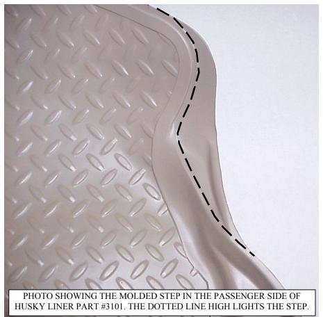
PHOTO SHOWING HUSKY LINER PART #3101 PASSENGER SIDE TRIMMED FOR USE IN VEHICLES WITH LARGE KICK PANEL.
