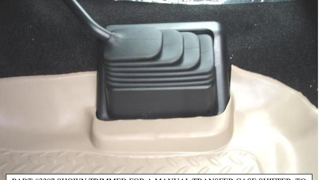
PART #3387 SHOWN TRIMMED FOR A MANUAL TRANSFER CASE SHIFTER. TO TRIM, SIMPLY REMOVE THE LOWERED SECTION ON THE LINER.
