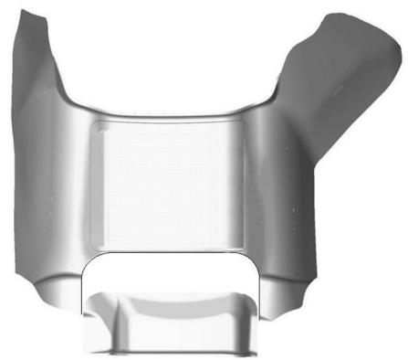
IF YOUR RAM TRUCK HAS THE STORAGE COMPARTMENT LOCATED ON THE TRANSMISSION TUNNEL IN FRONT OF THE CENTER SEAT, YOU WILL NEED TO TRIM YOUR CENTER HUMP LINER AS SHOWN ABOVE. TO TRIM, USE A PAIR OF HEAVY SHEARS OR A UTILITY KNIFE AND USE THE OFFSET IN THE LINER AS YOUR TRIMMING GUIDE.
