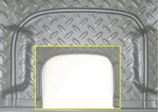
PART #6102 SHOWING THE TRIM AREA FOR A SECOND ROW CONSOLE EQUIPPED VEHICLE. NOTE THAT THERE IS A MOLDED IN GROOVE ALONG THE EDGE OF THE RAISED ROUND TO AID IN TRIMMING. THE PHOTO IN THE INSET SHOWS THE LINER TRIMMED.
