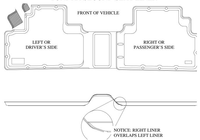
TUNDRA OWNERS WITH THE POWER SEAT OPTION WILL NEED TO TRIM THEIR DRIVER'S SIDE LINER TO ALLOW CLEARANCE OF THE POWER SEAT TRACK (SEE ABOVE). REMOVE THE MATERIAL FROM THE TWO RAISED AREAS. A UTILITY KNIFE OR SCISSORS WORK WELL.
