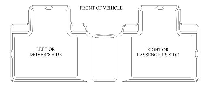
TO EASE INSTALLATION OF LINER, ADJUST BOTH FRONT SEATS TO THEIR MOST FORWARD POSITION AND FOLD SEATBACKS FORWARD BEFORE INSTALLING LINER. ONCE LINER IS INSTALLED, REPOSITION SEATS AS DESIRED.
