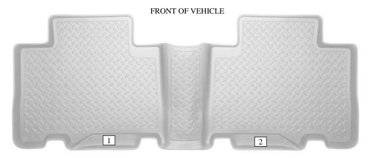
RAV4 LIMITED MODELS WITH  $3^{RD}$  ROW SEATING HAVE CLIMATE CONTROL DUCTING LOCATED ALONG THE REAR WALL OF THE  $2^{ND}$  ROW OF SEATS. THIS FEATURE KEEPS PART #6597 FROM FITTING CORRECTLY AS PACKAGED. HOWEVER, A TRIM AREA IS MOLDED INTO PART #6597 WHICH WILL ALLOW THIS PART TO BE TRIMMED TO ACCOMMODATE THE DUCTING. TO TRIM, REMOVE THE SECTIONS OF THE LINER SHOWN ABOVE LABELED #1 AND #2. USE THE MOLDED IN TRIM GROOVE AS YOUR TRIMMING GUIDE (SEE PHOTOS ON BACK).
