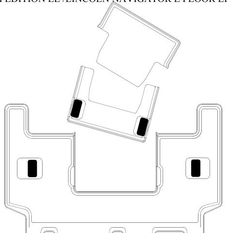
BEFORE INSTALLATION OF YOUR HUSKY LINER, CHECK LINER TO MAKE SURE THE FOUR (4) AREAS SHOWN ABOVE DARKENED ARE TRIMMED AWAY. IF THEY ARE NOT, DO NOT INSTALL LINER AS THE SECOND ROW OF SEATS WILL NOT LOCK SECURELY INTO POSITION. INSTEAD, PLEASE CALL HUSKY LINERS AT 800-344-8759.
