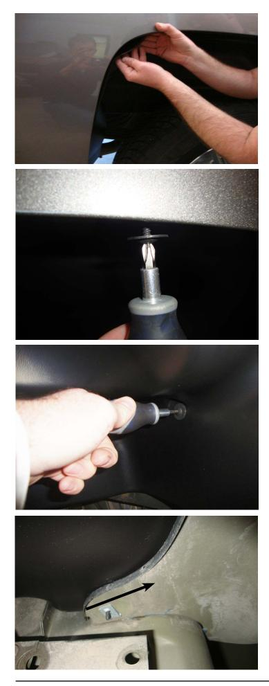
6. Tuck the remaining portion of the Wheel Well Guard behind the fender lip all the way around the fenderwell opening.
