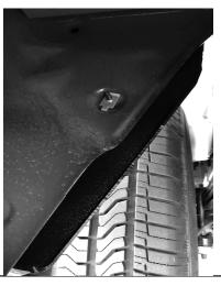
9. Align the 5 holes in the Wheel Well Guard with the factory screw locations and install the factory torx head screws. Install all screws before tighting.
