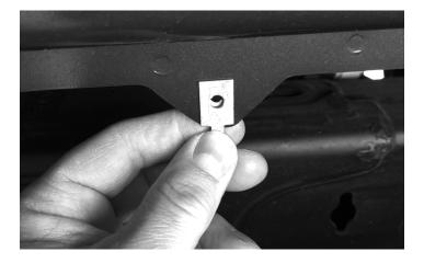
4. If your truck was not equipped with factory wheel well liners install a u-clip at locations B, C, and D by clipping the u-clip over the tab and aligning with the factory hole.
