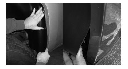
8. Insert the lower flap sections of the Wheel Well Guard into the fender well behind the fender well lip.
