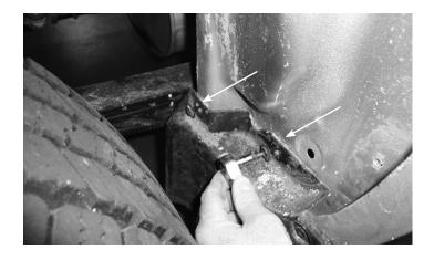
2. Reinstall 2 factory screws that hold the factory rock guard on the front/rear side of the fender and tighten.
