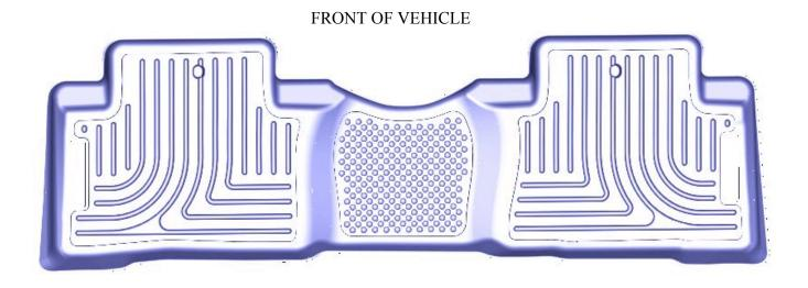
TO EASE INSTALLATION OF YOUR PILOT SECOND SEAT LINER, MOVE THE FRONT SEATS TO THEIR MOST FORWARD POSITIONS. WITH THIS DONE, INSERT LINER IN VEHICLE ANGLING IT SO THAT THE BACK EDGE OF THE LINER IS SEATED INTO PLACE FIRST, THEN LOWER FRONT PORTION. ONCE LINER IS INSTALLED, REPOSITION THE FRONT SEATS AS DESIRED.
