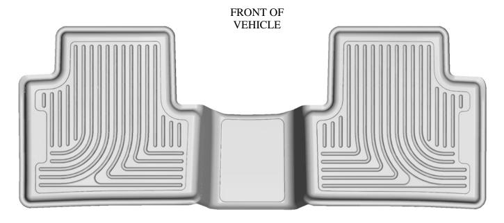
TO EASE INSTALLATION OF YOUR  $2^{\rm nd}$  SEAT FLOOR LINER, FIRST MOVE THE FRONT SEATS TO THEIR MOST FORWARD POSITIONS. WITH THIS DONE, INSERT LINERS IN VEHICLE THEN REPOSITION THE FRONT SEATS AS DESIRED.
