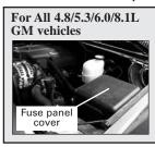
The fuse panel is located on the driver's side of the vehicle behind the vehicle battery. Lift off the cover to access the fuse block. You now can remove the fuse. To remove the fuse, hold the end of the fuse between your thumb and index finger and pull straight out. Make sure you remember to re-install the fuse in the proper location and re-install the fuse panel cover after programming your vehicle.
