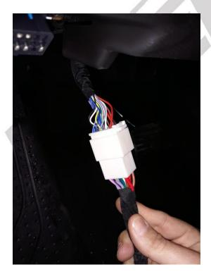
5. Plug the male end of the Speedometer Module Harness into the OE module and tuck the harness and Speedometer Module behind the kick panel.
