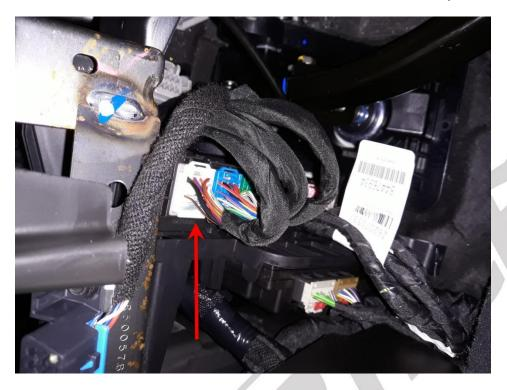
4. Plug the male end of the Inline Speedometer Module Harness into the female end of the OE Harness.
