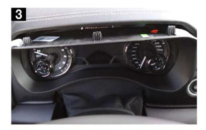
Lift out the rubber mat from the top of the instrument panel (touchscreen). Remove the two (2) screws. Some trucks require a T-20 torx driver while others require either a phillips head screwdriver or a 7mm socket.
