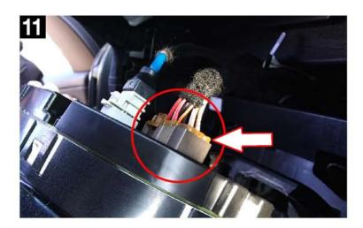
Insert the female end of the harness into the connector on the back of the instrument cluster (A). Then connect the black Molex connector to the Hypertech In-Line Speedometer Calibrator Module (B).
